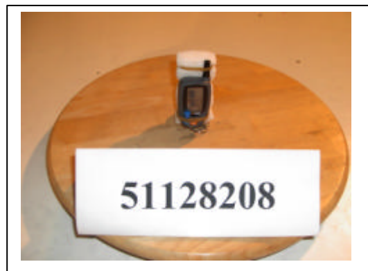
Radiated Open Site Test Set-up
