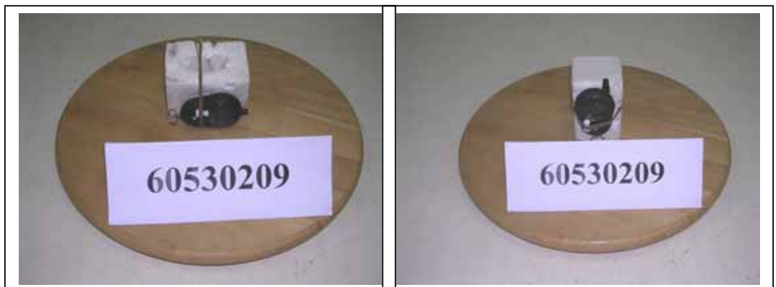
Radiated Open Site Test Set-up
