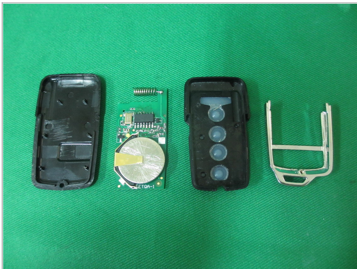
Inner View of EUT
