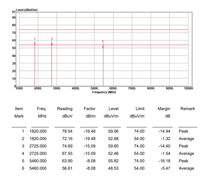
Remark: Corrected Level = Reading + Correction Factor - Preamp
