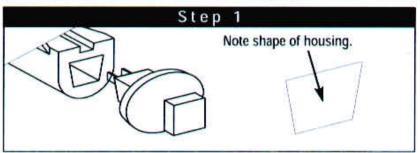
Insert the Valet Switch and Make Sure the Valet/Override Switch is in the "Off" Position
