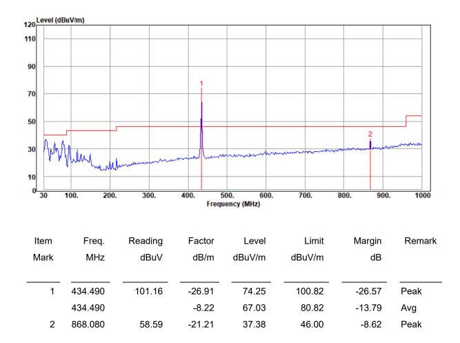
Remark : Corrected Level = Reading + Correction Factor – Preamp Correction Factor = Antenna Factor + Cable Loss Margin = Corrected Level – Limits " \* " Mark indicated Background Noise Level Avg Level=Peak Level – Factor CLIENT: Nutek Corporation EUT: Transmitter
