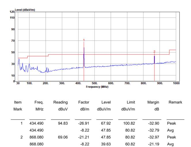
Remark : Corrected Level = Reading + Correction Factor – Preamp Correction Factor = Antenna Factor + Cable Loss Margin = Corrected Level – Limits "\*" Mark indicated Background Noise Level Avg Level=Peak Level – Factor
