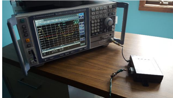
Figure 5: Conducted RF Test Setup Photograph(s).
