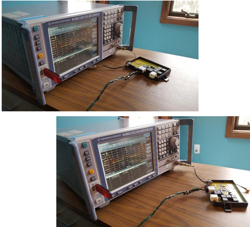
Figure 5: Conducted RF Test Setup Photograph(s).
