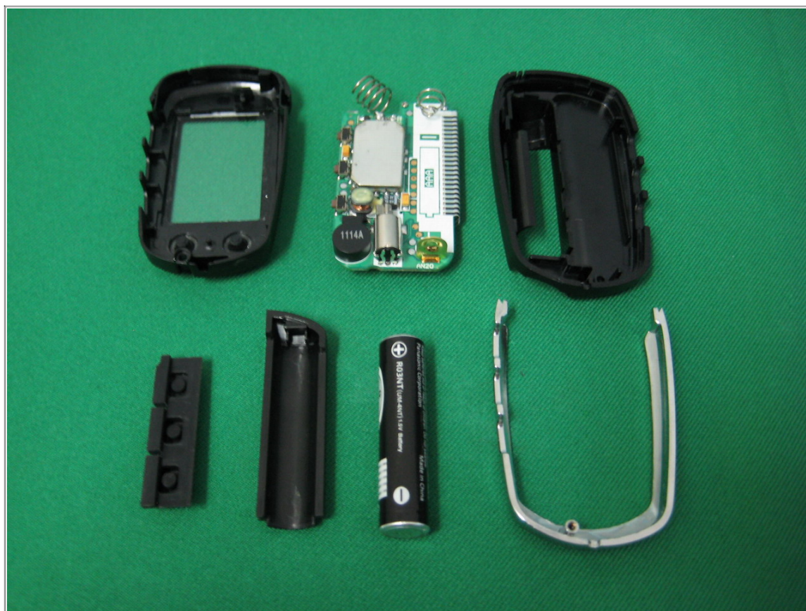
Inner View of EUT
