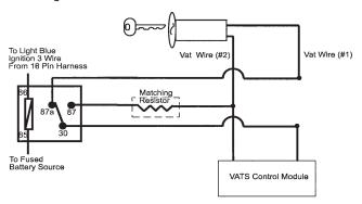
**Note:** For Hybrid mode, Bank 3 feature selection 5, this connection is not used, the unit will start the vehicle and run the allotted time based on feature selection and crank duration.
