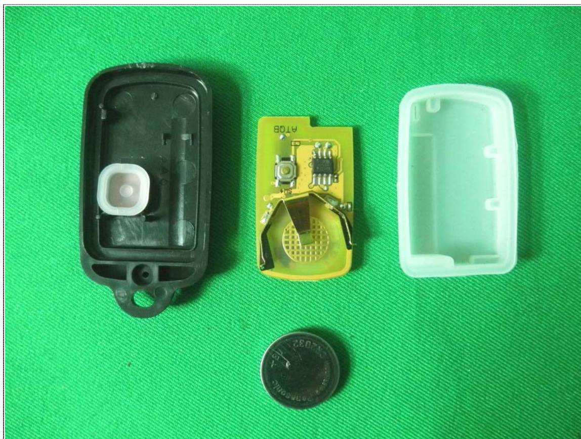
Inner View of EUT
