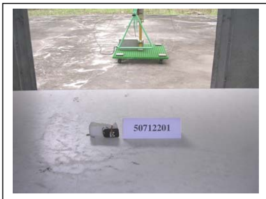
Radiated Open Site Test Set-up
