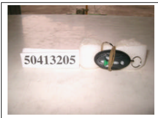
Radiated Open Site Test Set-up
