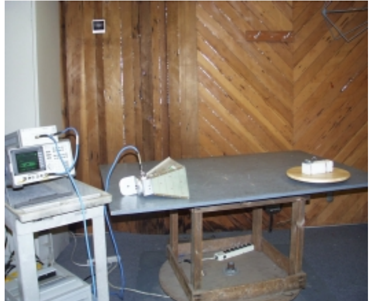
Radiated Open Site Test Set-up
