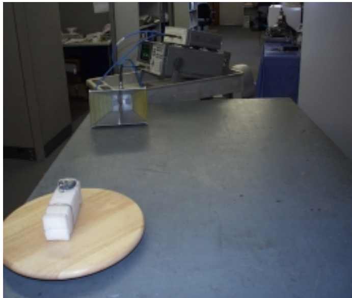
Radiated Open Site Test Set-up
