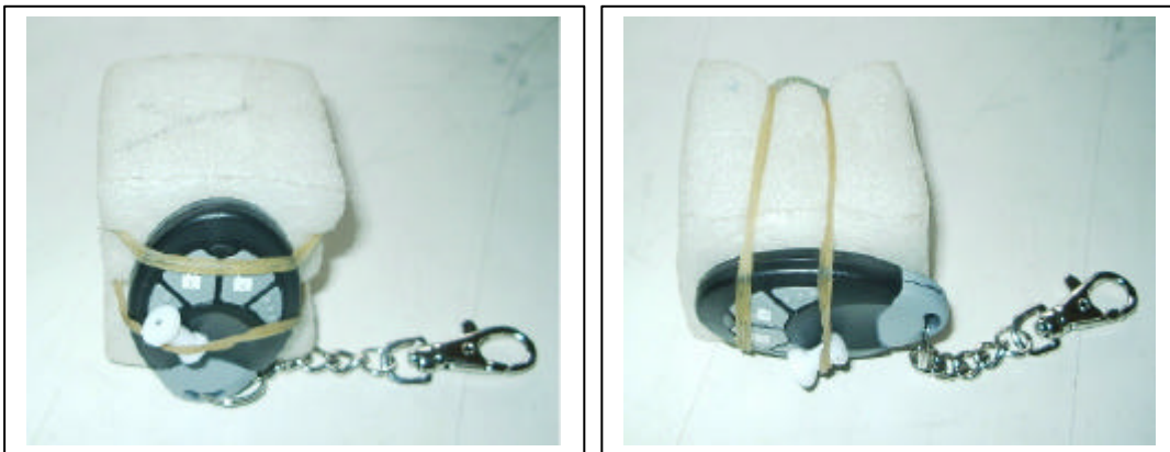
Radiated Open Site Test Set-up
