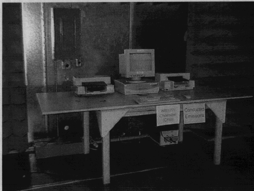
Conducted Emissions, Test Setup.
