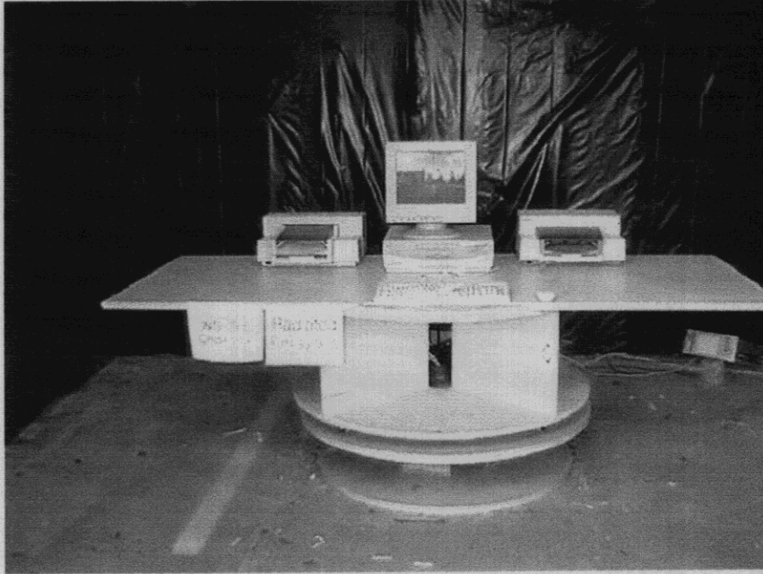
Radiated Emissions, Test Setup.
