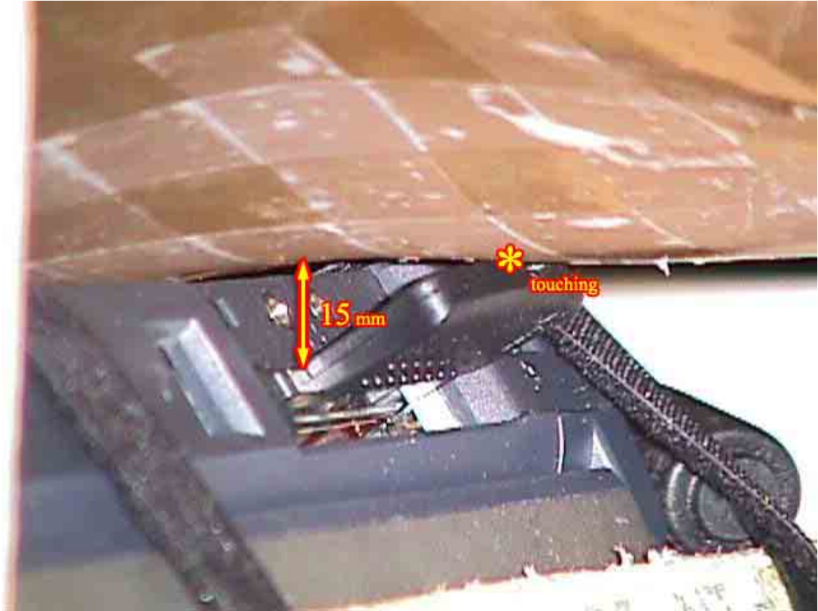
< Close-up view – Waist with the tip of EUT in contact with the phantom and the front of EUT faced outward from the phantom >
