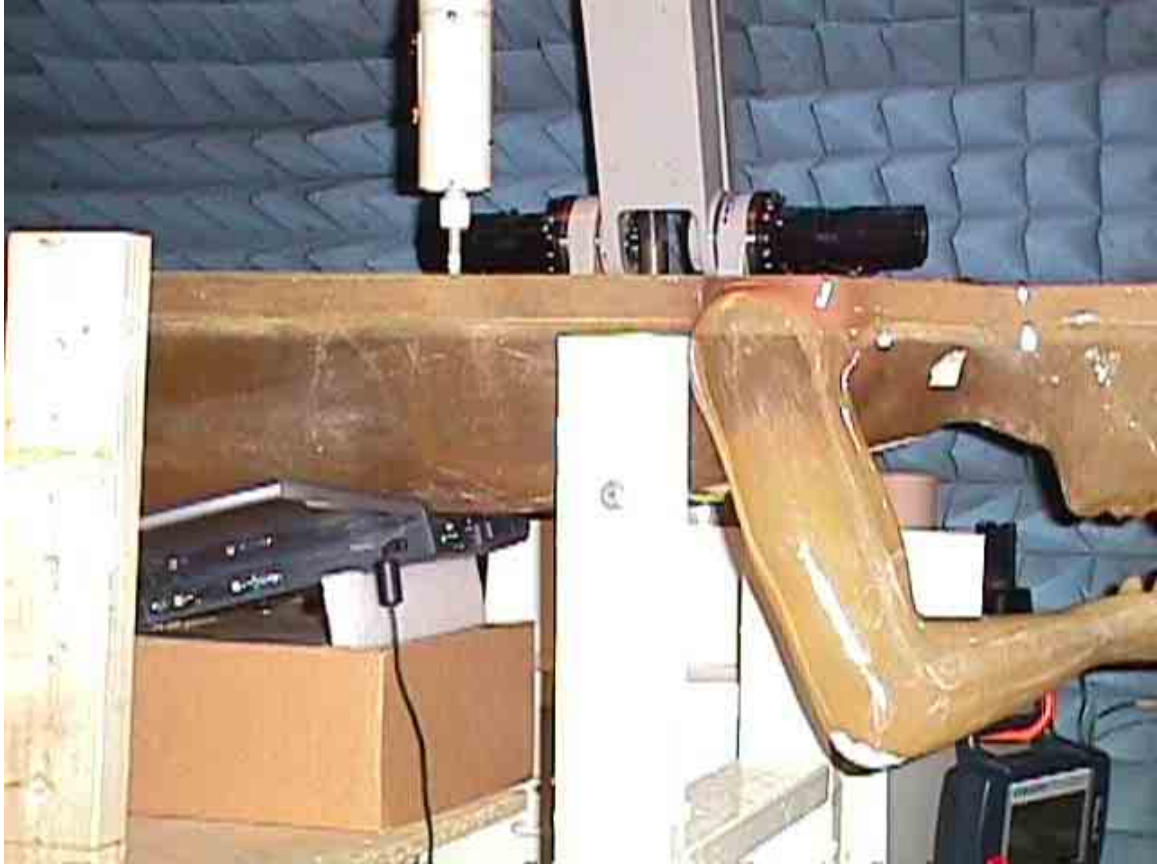
< Overview – Waist with the tip of EUT in contact with the phantom and the front of EUT faced inward to the phantom >
