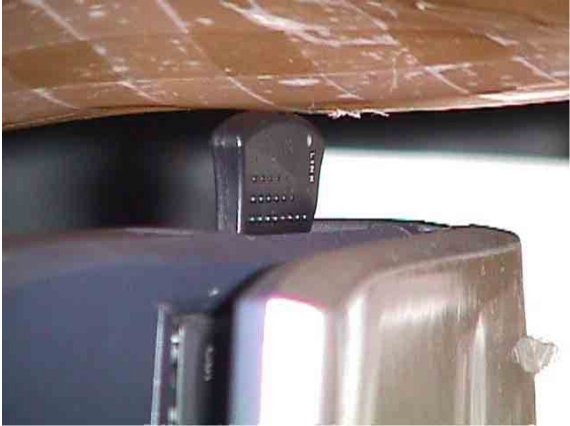
< Close-up view – Waist with the tip of EUT in contact with the phantom and EUT normal to the phantom >
