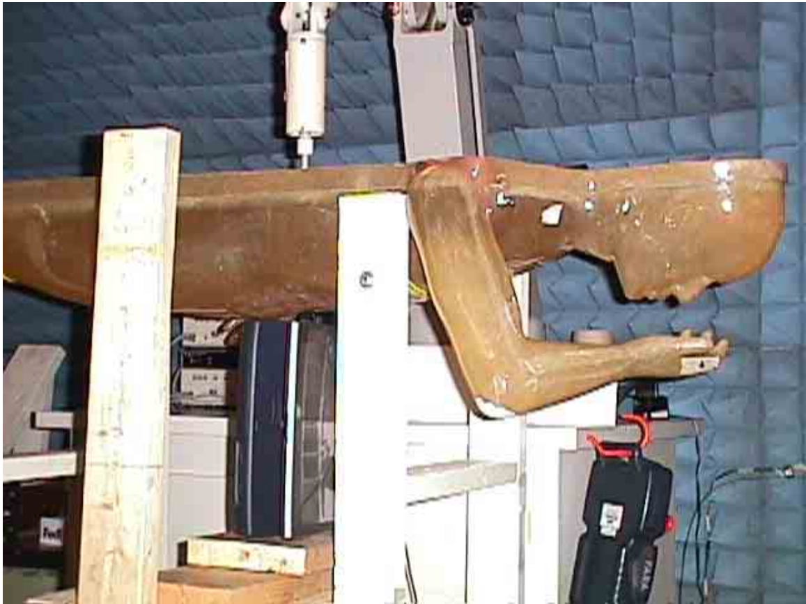
< Overview – Waist with the tip of EUT in contact with the phantom and EUT normal to the phantom >
