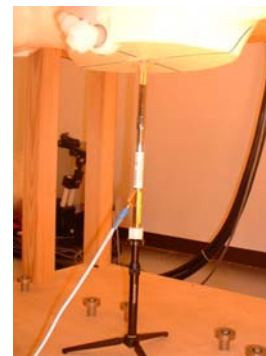
2450MHz System performance check setup
