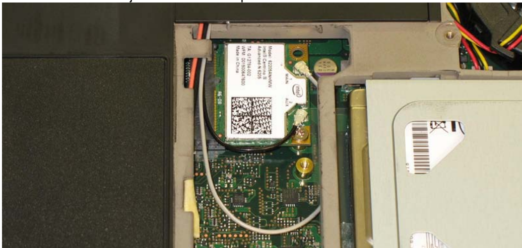
62205ANHMW inside the Fujitsu TABLET Computer
