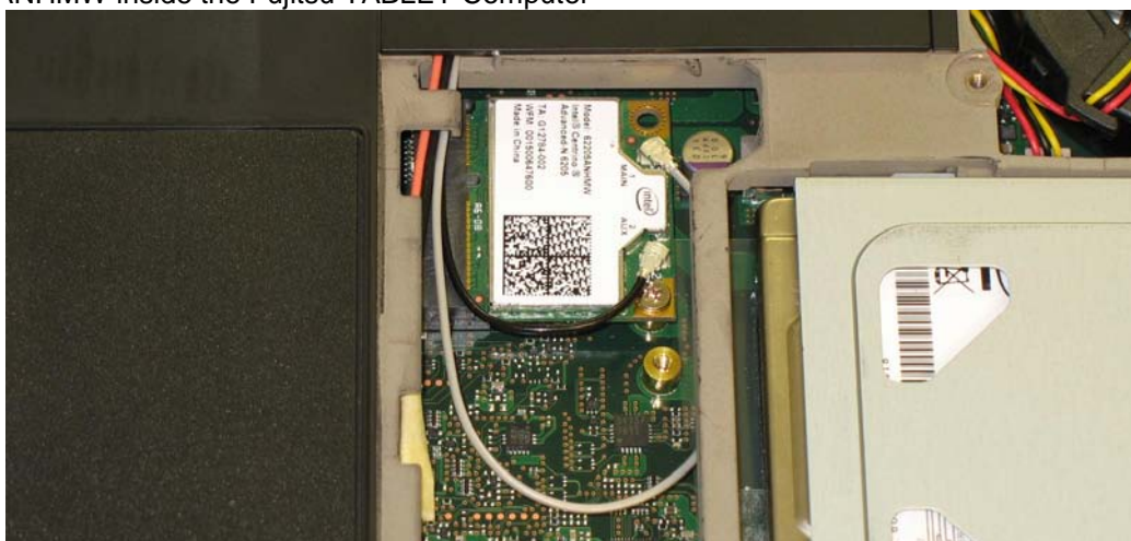
62205ANHMW inside the Fujitsu TABLET Computer
