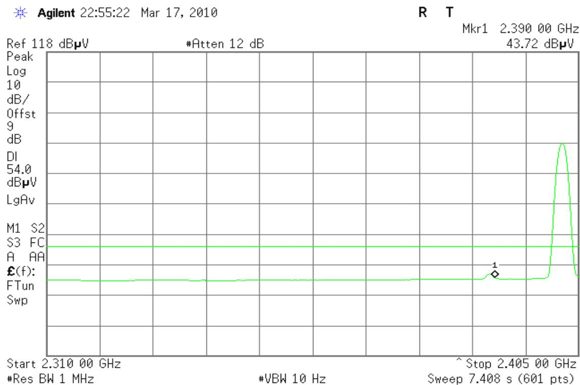
**Band Edges (CH High)****Detector mode: Peak****Polarity: Vertical**
