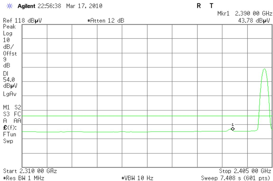
**Band Edges (CH High)****Detector mode: Peak****Polarity: Vertical**
