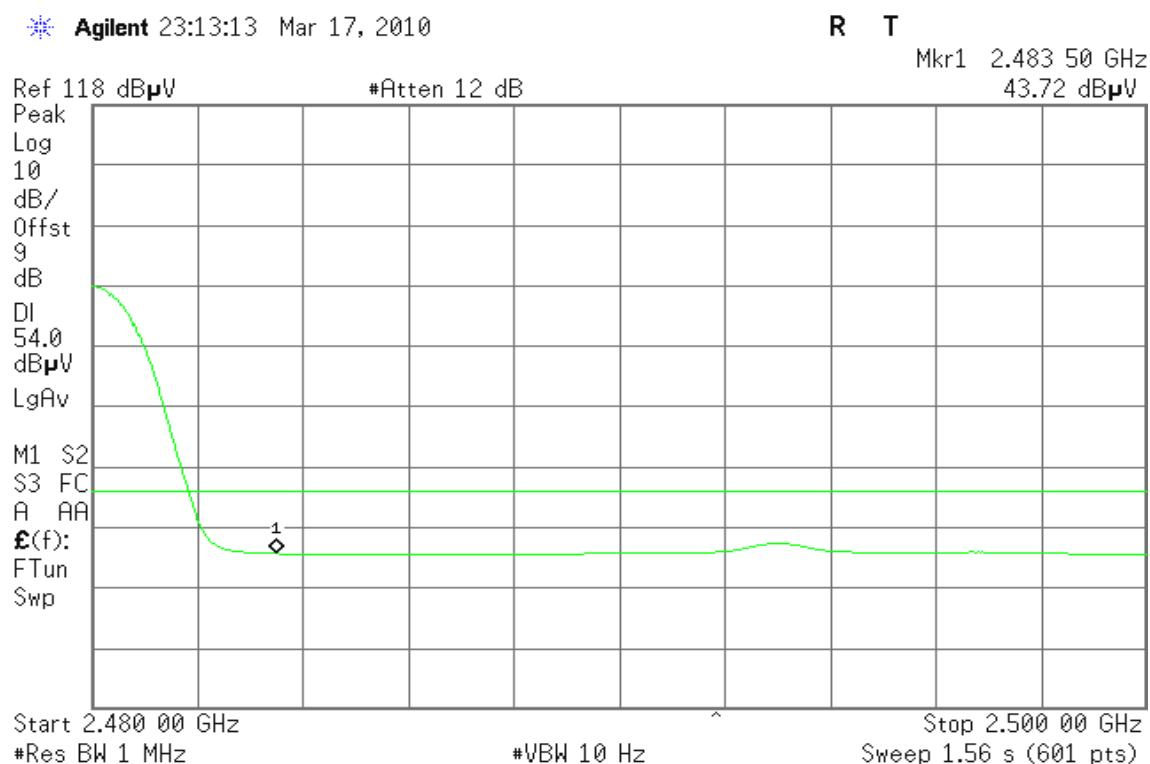
**For 8DPSK / DH5****Band Edges (CH Low)****Detector mode: Peak****Polarity: Vertical**
