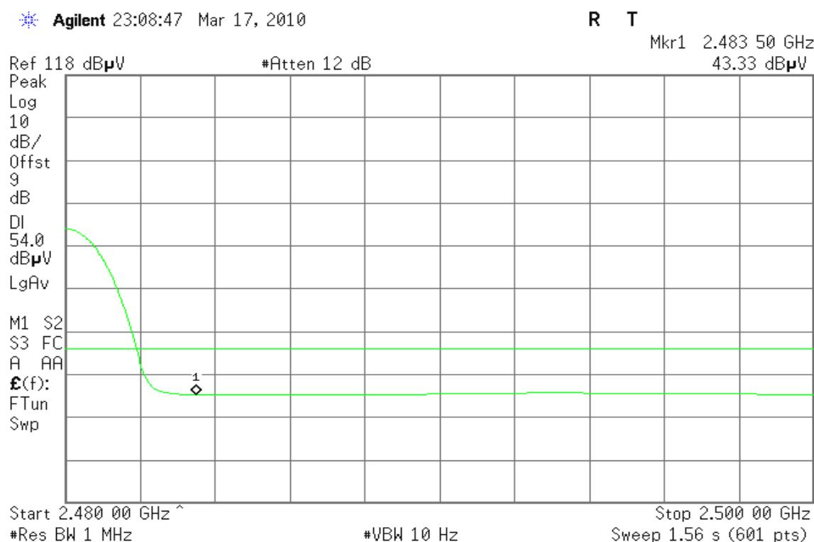
**Detector mode: Peak****Polarity: Horizontal**
