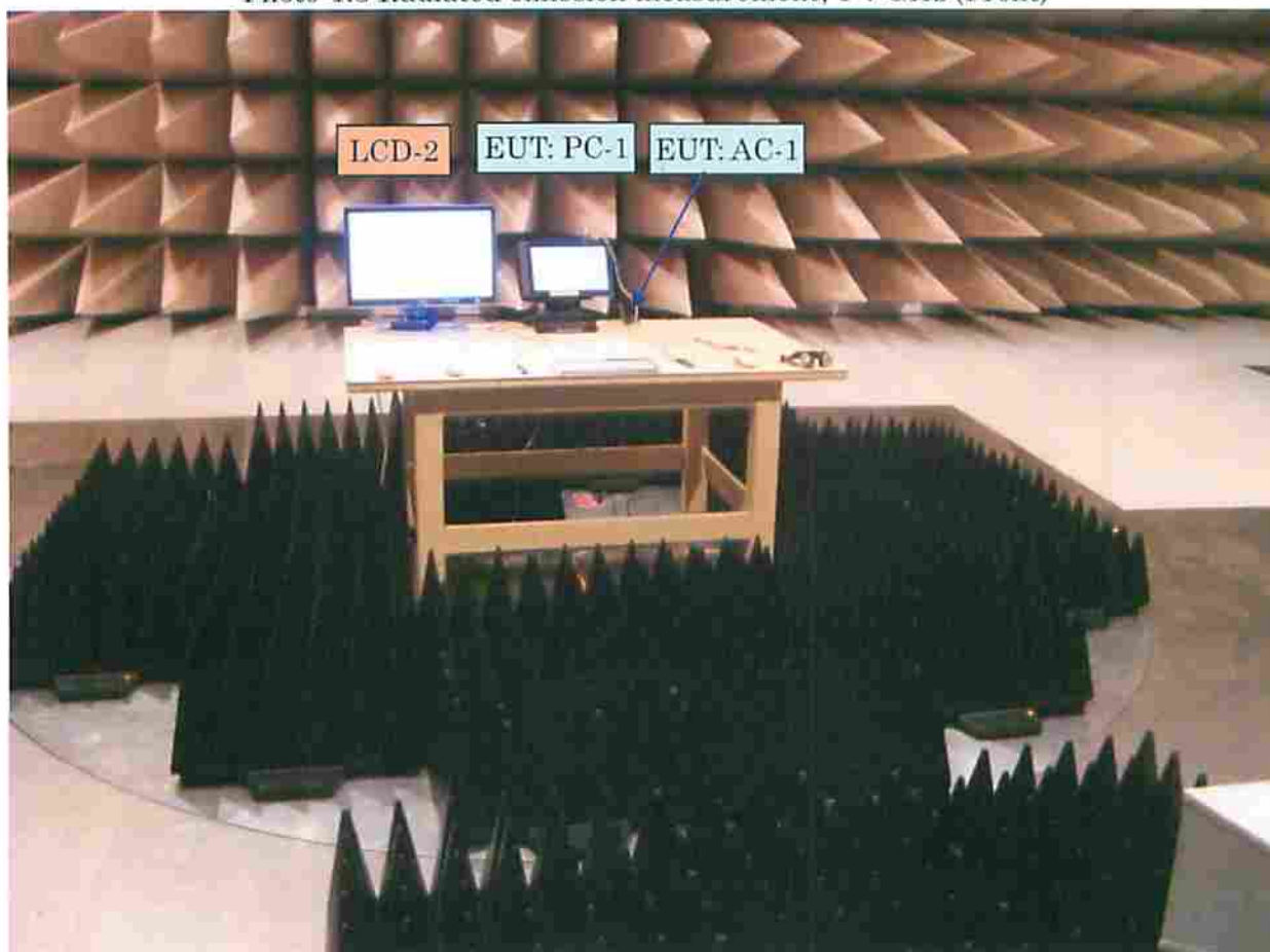
Photo-1.3 Radiated emission measurement; 1-7 GHz (Front)
