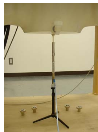
5100-5800MHz System performance check setup
