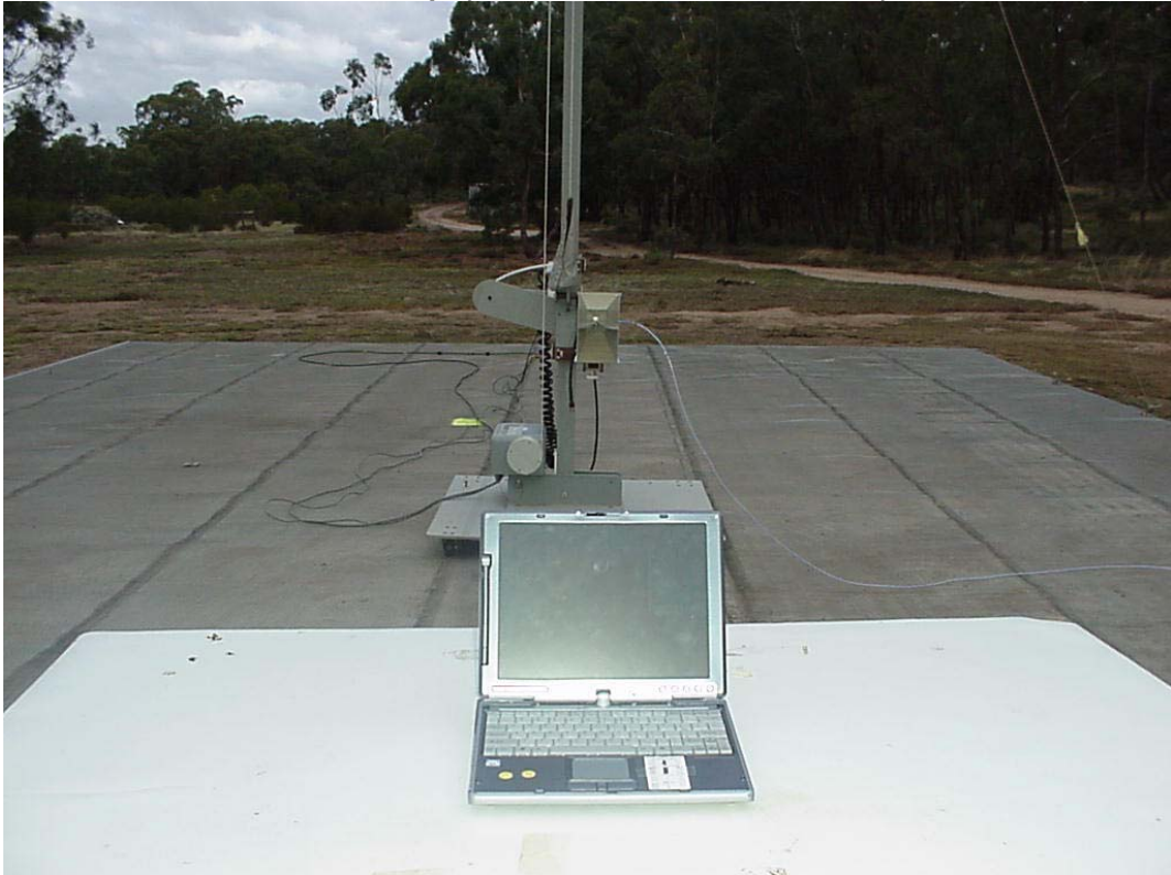
Radiated Emissions Test Setup (3 metre distance - Harmonics)
