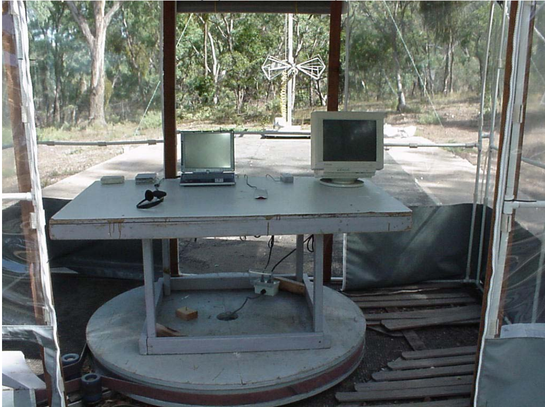
Radiated Emissions Test Setup (10 metre distance)
