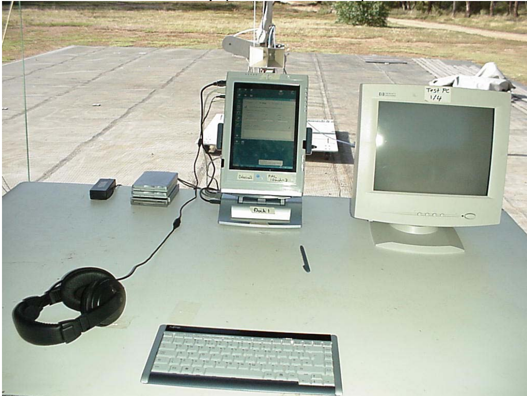
Peak Output Power, Spectral Density, Bandwidth and Band Edge Test Set Up.
