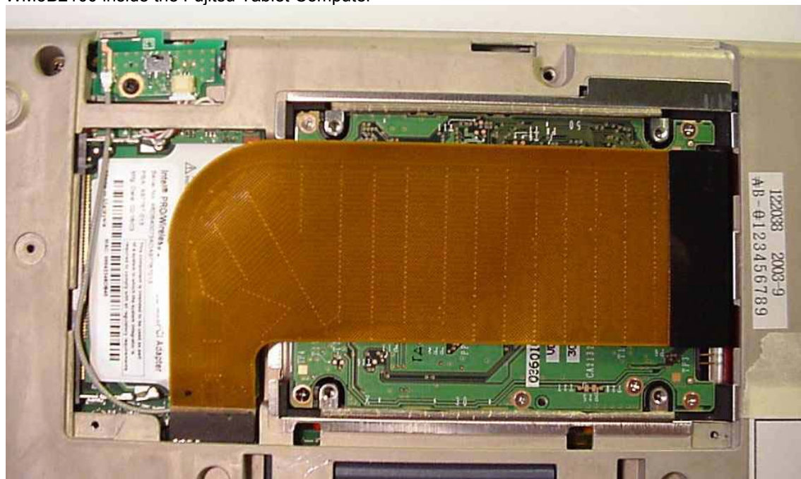
WM3B2100 inside the Fujitsu Tablet Computer
