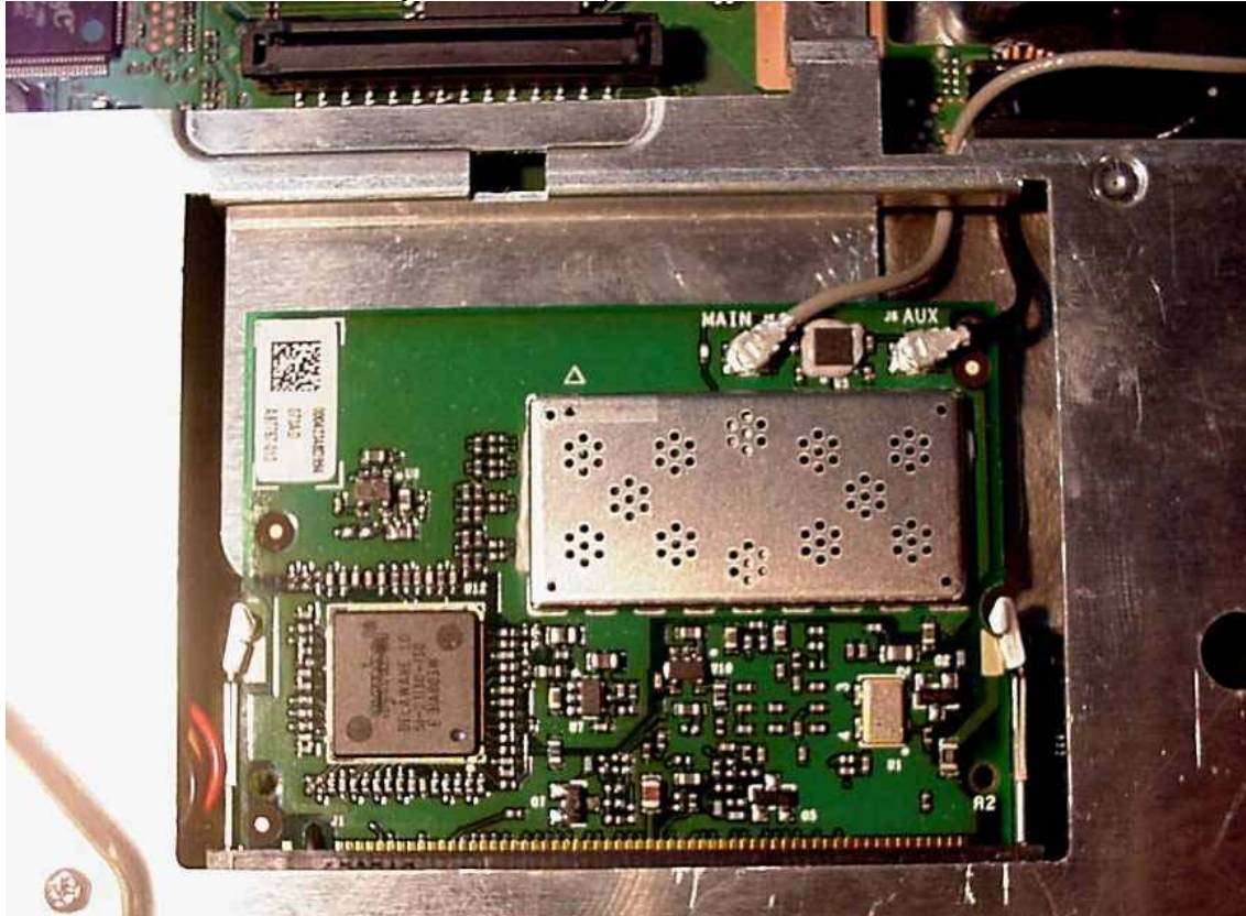
WM3B2100-MACE inside the Fujitsu Tablet Computer
