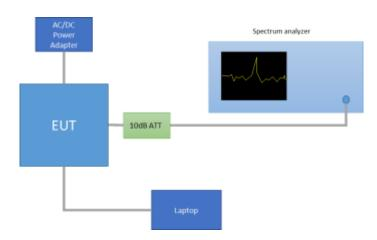
For the overlapped channels between U-NII-2C and U-NII-3, and according to FCC KDB 644545 D03, the power is computed based on the portion of the emission bandwidth (26dB) contained within that band. This rule is only applicable for those channels marked as overlapped.
