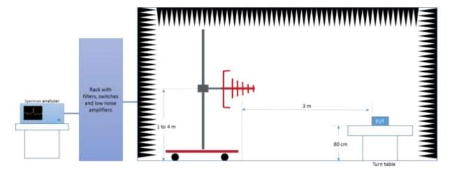
Radiated Setup 1 GHz - 18 GHz
