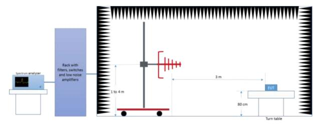
Radiated Setup 1 GHz - 18 GHz
