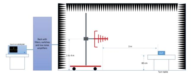
Radiated Setup 1 GHz - 18 GHz
