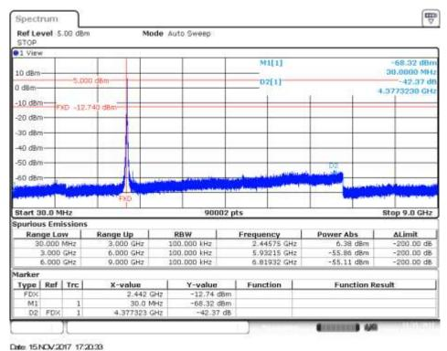
Channel 7 - Spurious 2 Delta Marker Measurement
