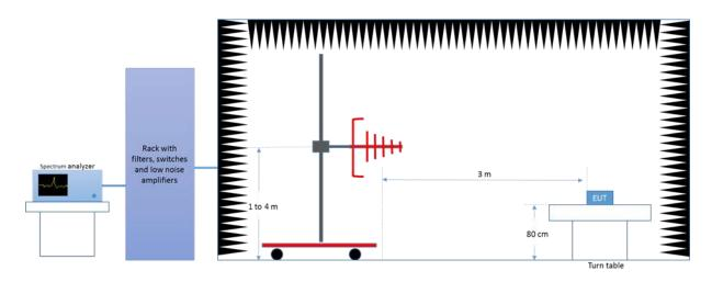
Radiated Setup 1 GHz – 18 GHz
