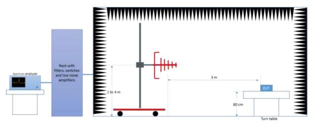
Radiated Setup 1 GHz - 18 GHz
