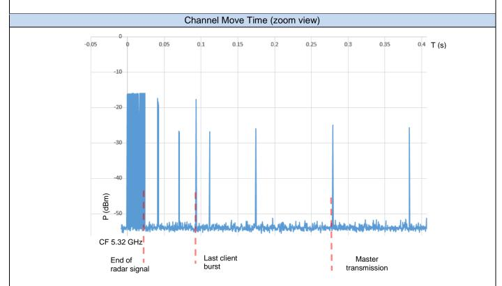
This zoom picture is generated with MS Excel using post processing of the sampling trace.
