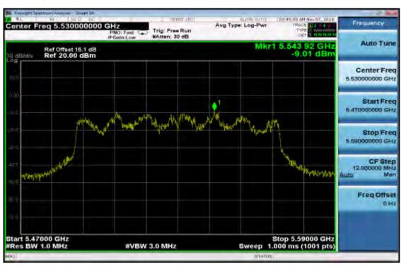
Peak Power Spectral Density Data Plot (CH Low 5610 MHz)
