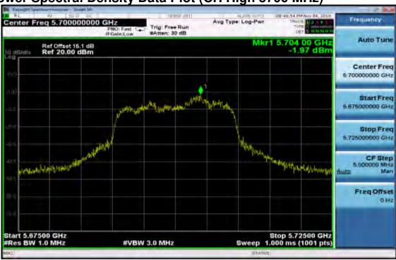
802.11n HT20, 5470~5725 MHz Peak Power Spectral Density Data Plot (CH High 5720 MHz)
