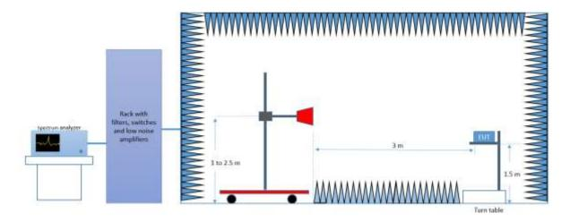
Radiated Setup 18 GHz - 26.5 GHz
