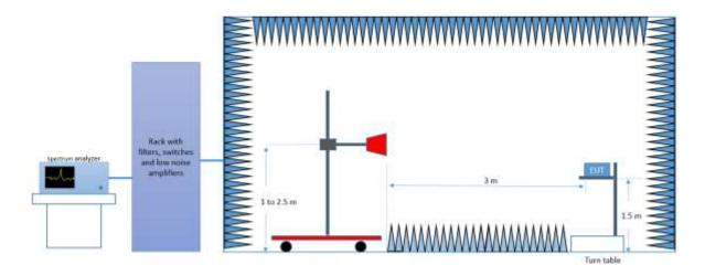
Radiated Setup 18 GHz - 26.5 GHz
