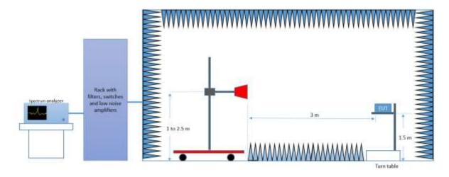
Radiated Setup 18 GHz - 26.5 GHz
