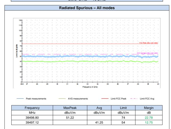
Note 1: The spurious signals detected do not depend on either the operating channel or the modulation mode.
