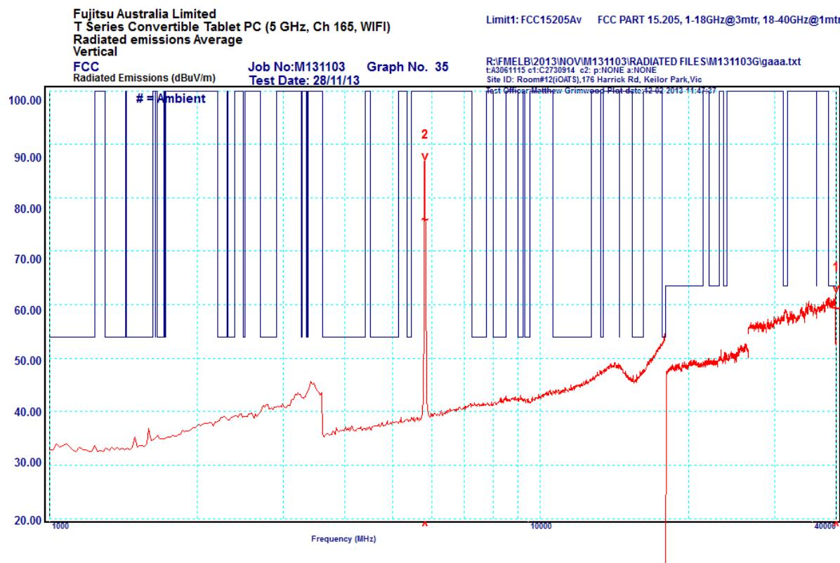
**Result:** Harmonics and spurious emissions were investigated between 1 and 40 GHz. Other emissions were confirmed low with both RBW and VBW reduced. The worst case emissions complied with the FCC limits of sections 15.209 and 15.247.
