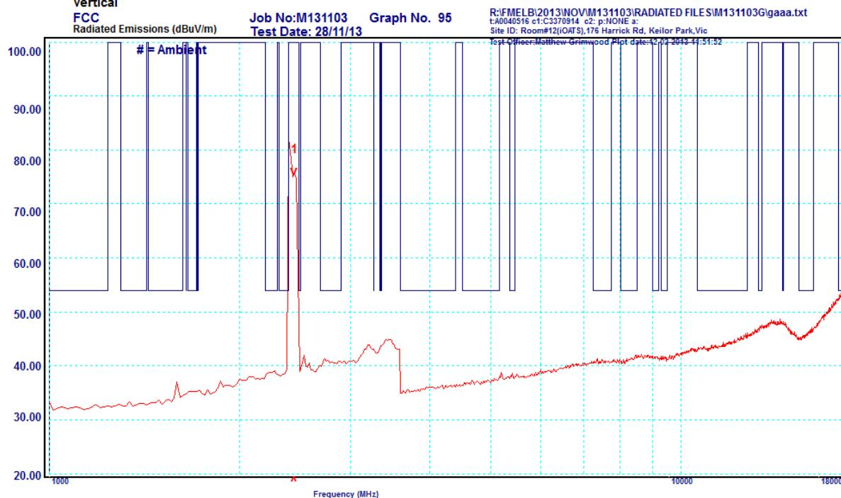
**Result:** Harmonics and spurious emissions were investigated between 1 and 25 GHz. Other emissions were confirmed low with both RBW and VBW reduced. The worst case emissions complied with the FCC limits of sections 15.209 and 15.247.
