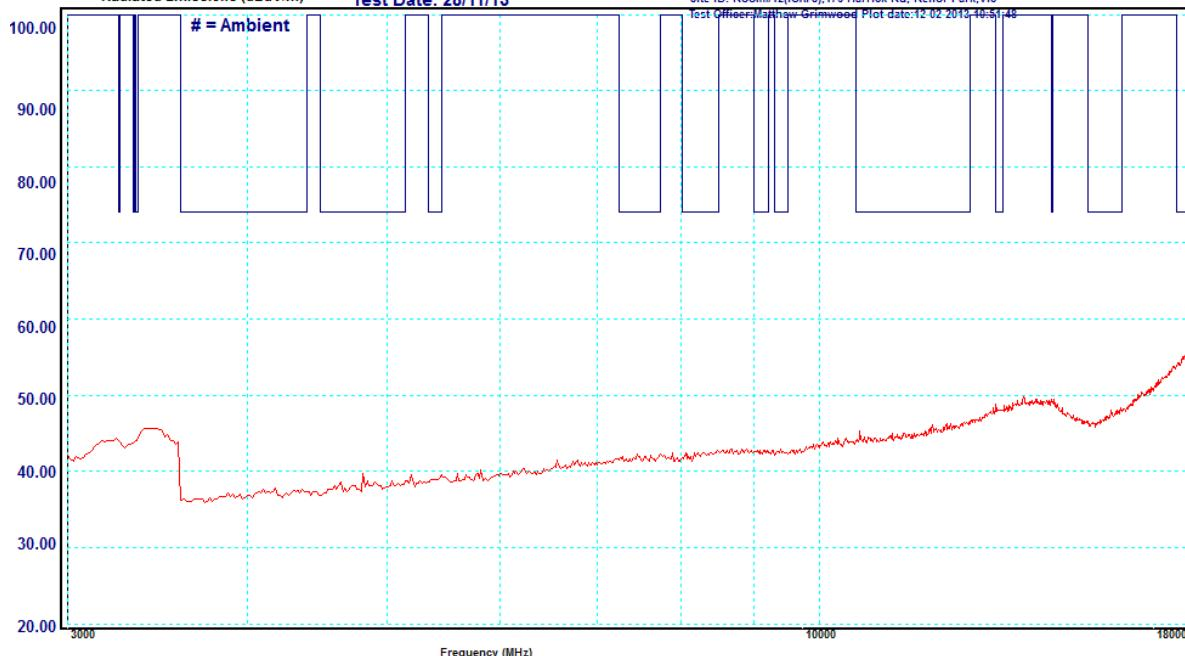
**Result:** Harmonics and spurious emissions were investigated between 1 and 25 GHz. Other emissions were confirmed low with both RBW and VBW reduced. The worst case emissions complied with the FCC limits of sections 15.209 and 15.247.
