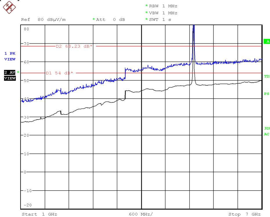
Note: The peak above the limit is the carrier frequency. This plot is valid for Chain A, Chain B and Chain A+B.
