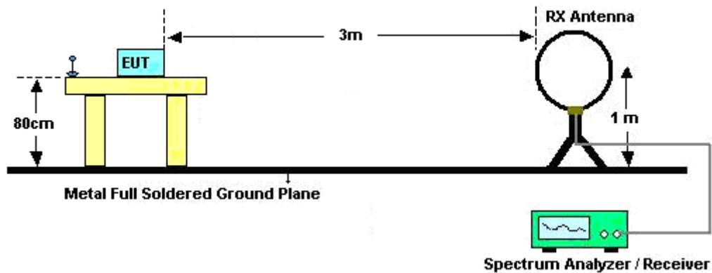
For radiated emissions from 30MHz to 1GHz
