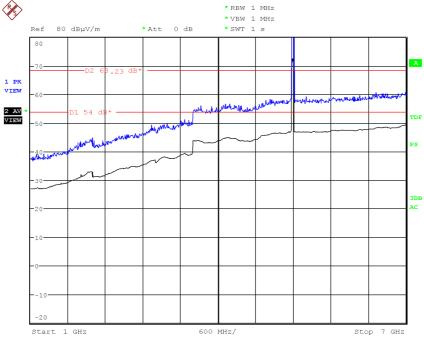
The peak above the limit is the carrier frequency. This plot is valid for Chain A, Chain B and Chain A+B.
