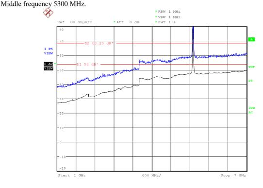
Note: The peak above the limit is the carrier frequency. This plot is valid for both Chain A and Chain B.
