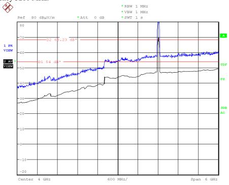
The peak above the limit is the carrier frequency. This plot is valid for Chain A, Chain B and Chain A+B.
