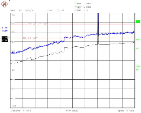
Note: The peak above the limit is the carrier frequency. This plot is valid for both Chain A and Chain B.
