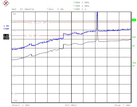
Note: The peak above the limit is the carrier frequency. This plot is valid for Chain A, Chain B and Chain A+B.
