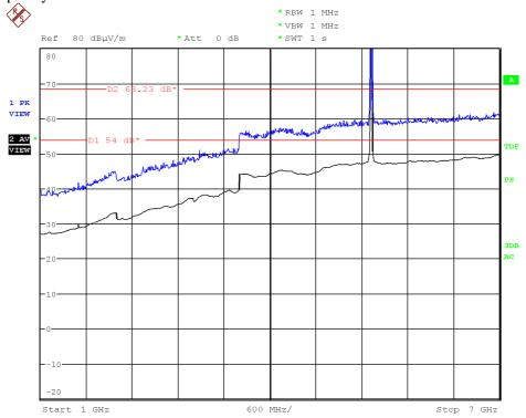
Note: The peak above the limit is the carrier frequency. This plot is valid for both Chain A and Chain B.
