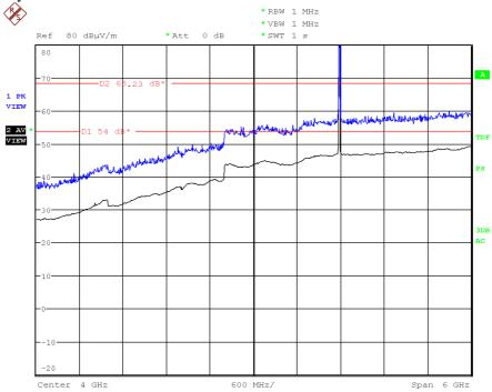
Note: The peak above the limit is the carrier frequency. This plot is valid for both Chain A and Chain B. Middle frequency 5200 MHz.
