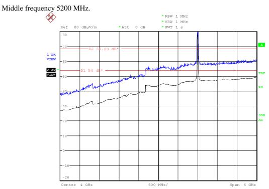
The peak above the limit is the carrier frequency. This plot is valid for Chain A, Chain B and Chain A+B.
