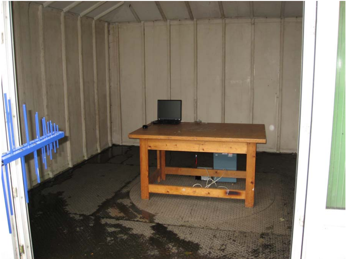
Photograph 1: Test setup radiated emissions - front
