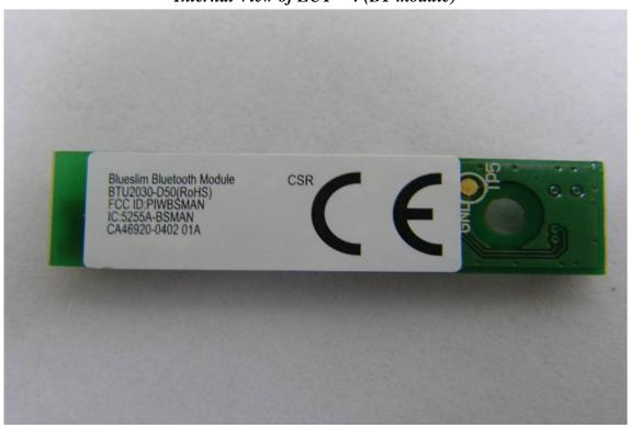
Internal View of EUT – 5 (BT module)
