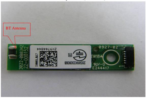
Internal View of EUT – 3 (BT module)
