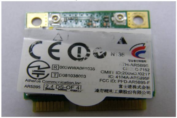
Internal View of EUT – 7 (WLAN Module)
