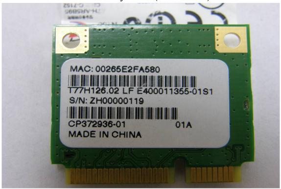
Internal View of EUT – 9 (WLAN Module)
