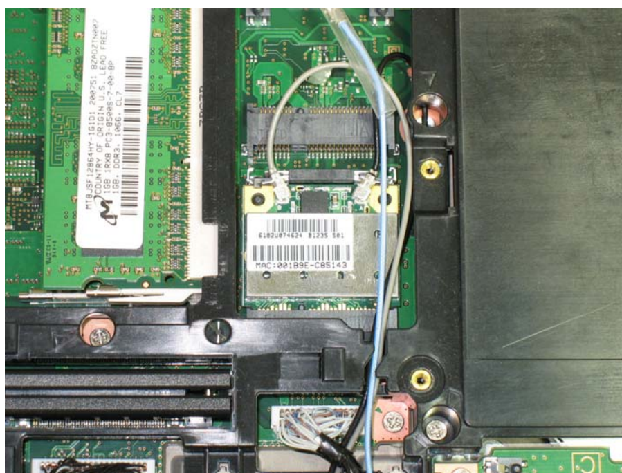
Model: AR5BHB92 (Atheros WLAN Module) inside the Fujitsu Portable Tablet Computer
