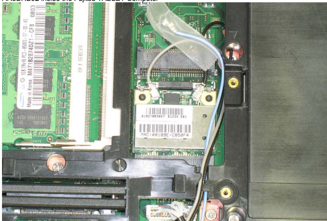
AR5BHB92 inside the Fujitsu TABLET Computer
