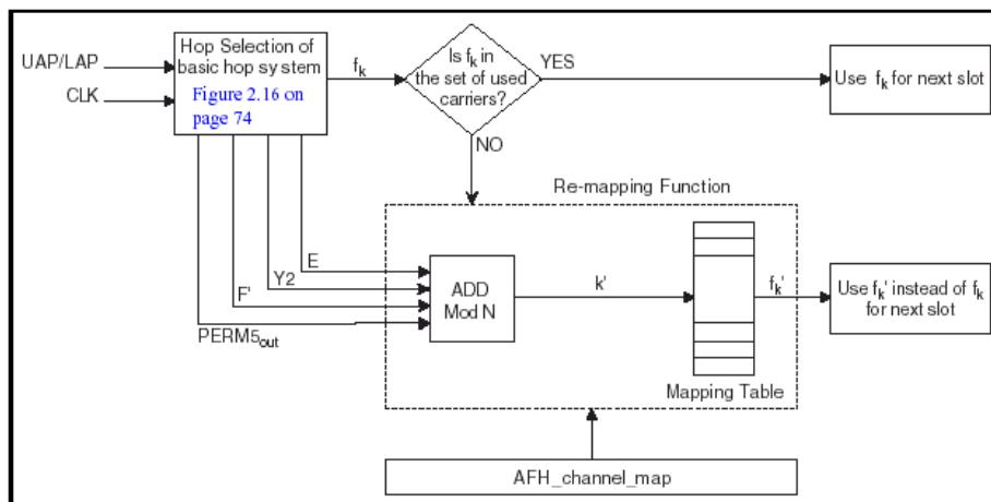
Also in the case of AFH, the fundamental sign adopt the sign head 160 that is the same as the case of 79Hopping. Hopping Pattern uses the value that is worked out by dividing with the number of AFH-Channel's. Then, available Hopping becomes even as well as 79Hopping.
