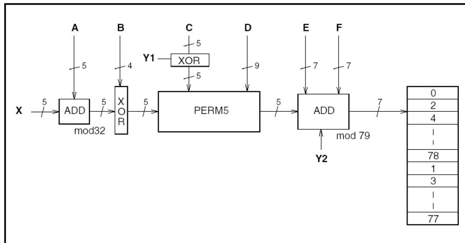
Due to the above flow, 32 hops are made into 5 ways. Then, the sign of the sign head 160 is formed. The remainder that is worked out by dividing with 79 is assigned to Hopping Channel.
