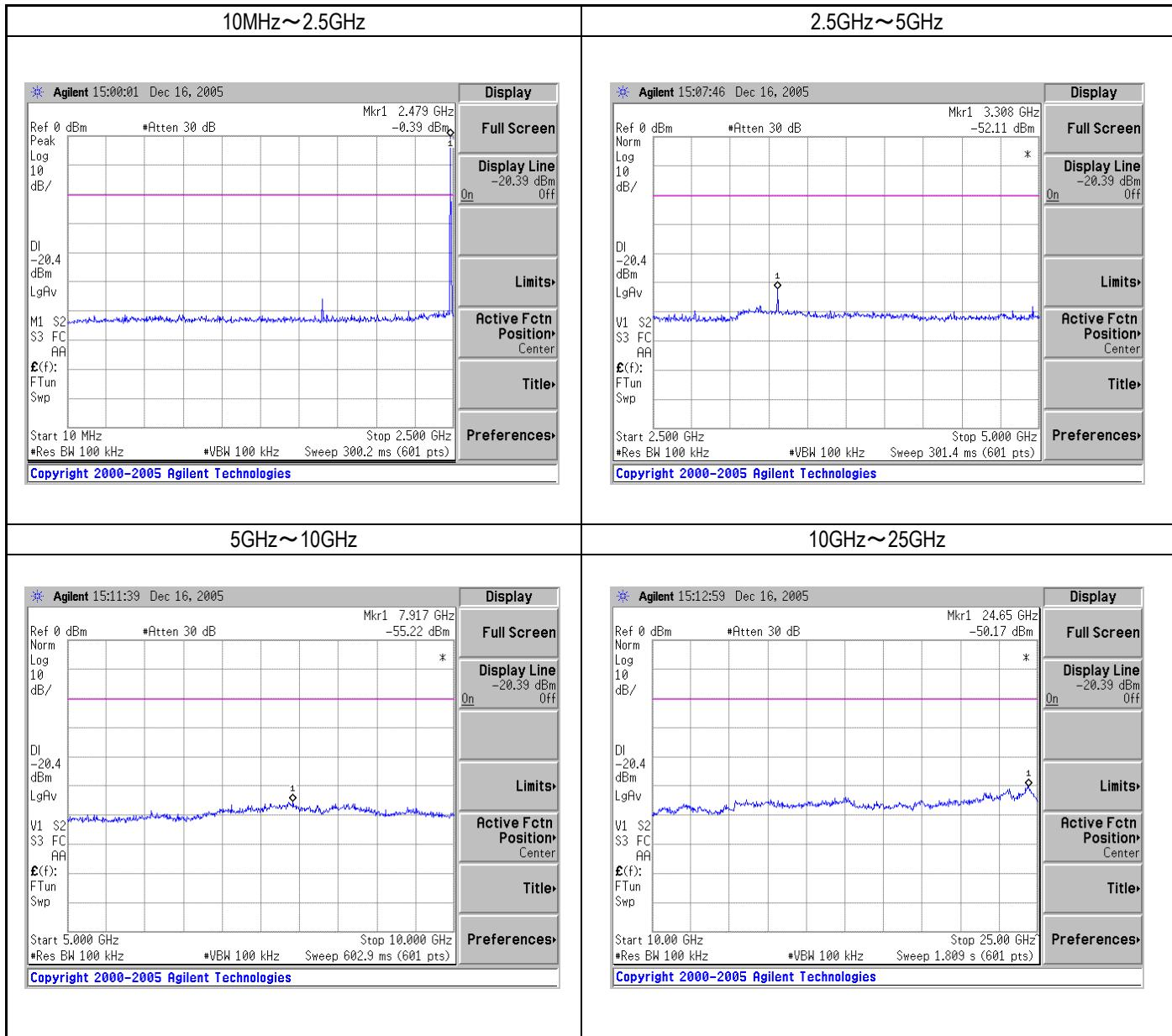
The spectrum data are attached below. Display line indicates the 20dB offset below highest level.
