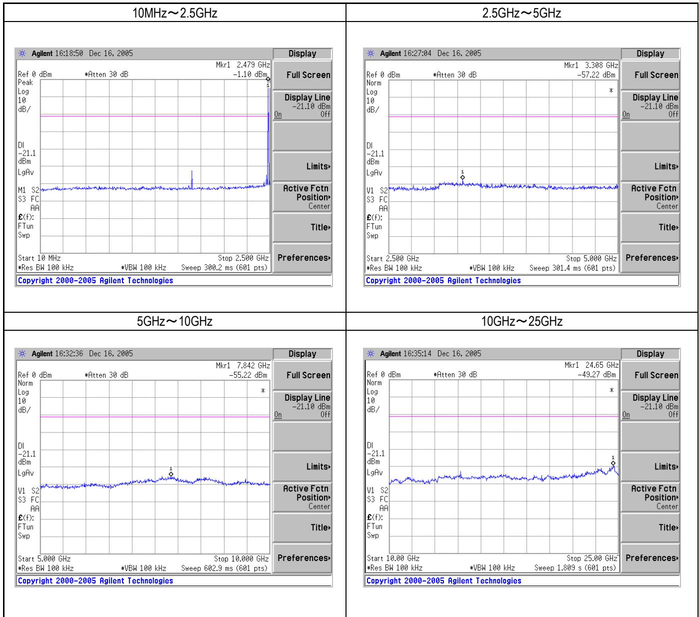
The spectrum data are attached below. Display line indicates the 20dB offset below highest level.
