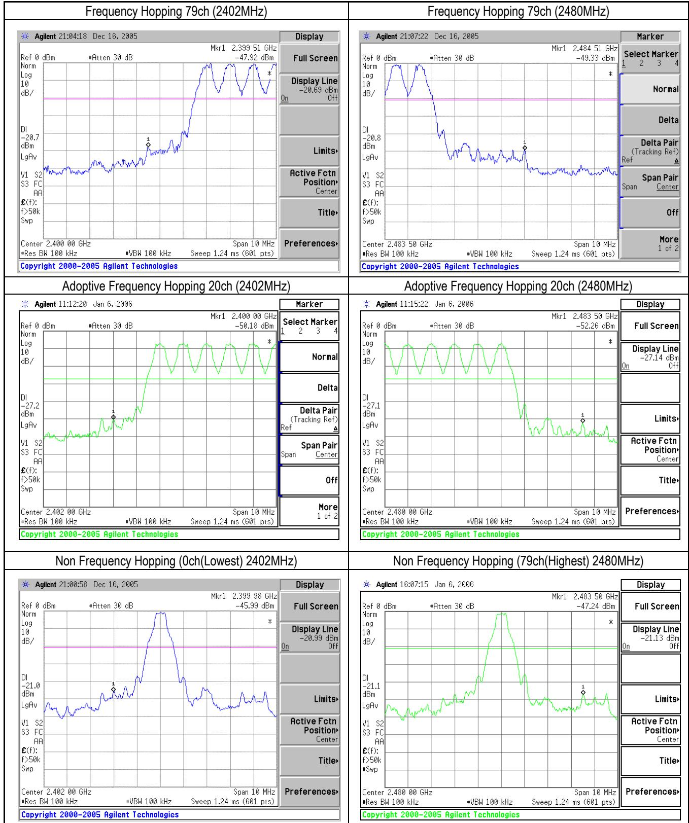
(2) Operation mode: Transmitting mode ( $\pi/4$  DQPSK Modulation)
