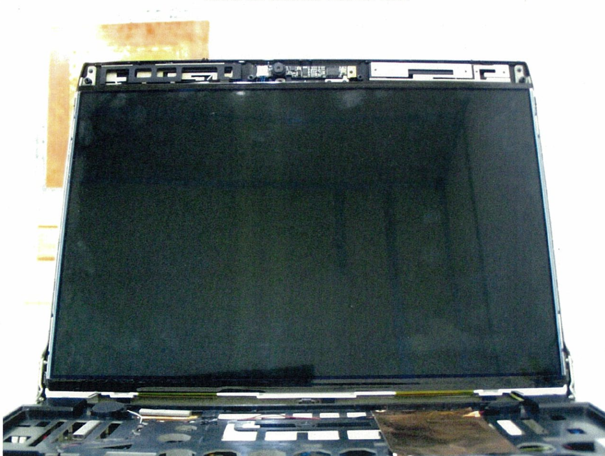
Photo-4.1 Internal view for LCD
