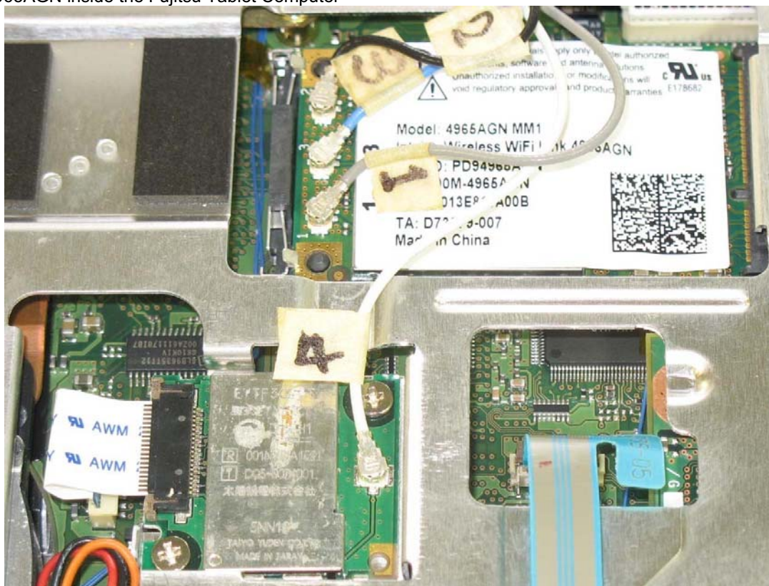
4965AGN inside the Fujitsu Tablet Computer
