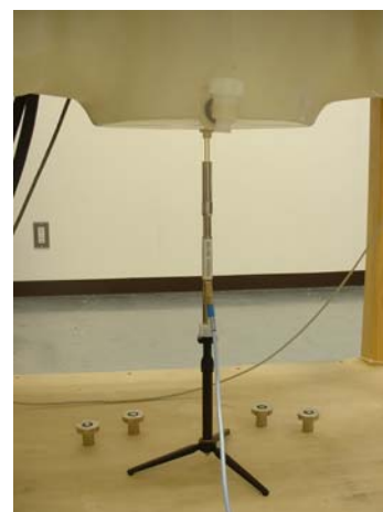
5100-5800MHz System performance check setup
