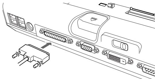
**Figure 4-17. Connecting a Parallel Device to Port Replicator****SERIAL PORT**
