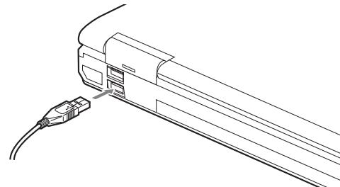
**Figure 4-19. Connecting a USB Device****INFRARED PORT**
