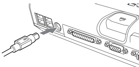
**Figure 4-18. Connecting a PS/2 Device****DOCKING PORT**
