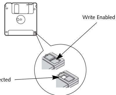
Figure 4-5. Floppy Disk Write Protect
