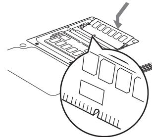
Figure 4-8. Installing a Second Memory Module
