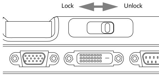
**Figure 4-14. Locking the Port Replicator****DETACHING THE PORT REPLICATOR**
