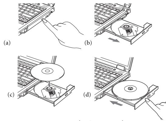
Figure 4-3. Loading/Ejecting Media
